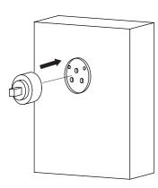
Use allen wrech to fix the HEX screw tightenly
