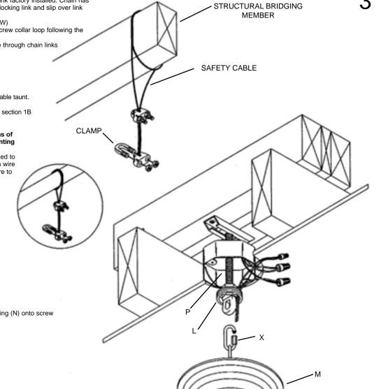
NOTE: NEC CODE (314.24) requires that ceiling outlet boxes in the United States support up to 50 lbs. This fixture exceeds 50 lbs. and must be installed using an outlet box approved for up to 100 lbs. or independently of the existing outlet box. Installation hardware and instructions are provided for both.
