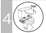
Mount bidet and toilet seat/lid over toilet mounting holes. Supplied rubber O-rings should be placed under the bidet mounting bracket to protect and secure bidet on the toilet.
