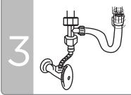
Connect supplied T valve to the toilet fill valve. Note T valve will be connected directly to toilet fill valve, not the shut off valve. Then connect rest of water lines to connected T valve.
