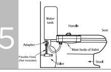
Open shut off valve and check for any leaks.
