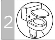
Remove existing seat and lid. Release the bolts on both side of the existing toilet seat.
