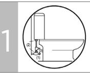
Shut water supply by turning it to the right and disassemble the water hose. Flush toilet to drain water inside
