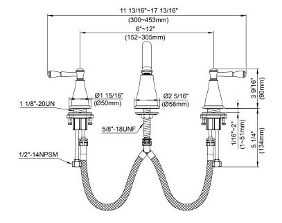
\* Installation method shown is for deck thickness of less than 1". If the installation is for deck thickness between 1" and 2", the sleeve nut needs to be reversed.
