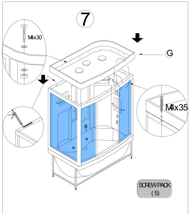
Put the roof onto the cabins and join the connection with sealant or sealant strip. And fasten with M4x35mm and M4x30mm screw.
