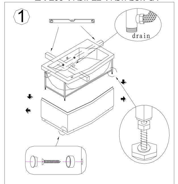
Remove the skirt fist, Connect the drain pipe. Adjust the cabinet with gradienter to the certain high. To be sure the whole unit is level.
