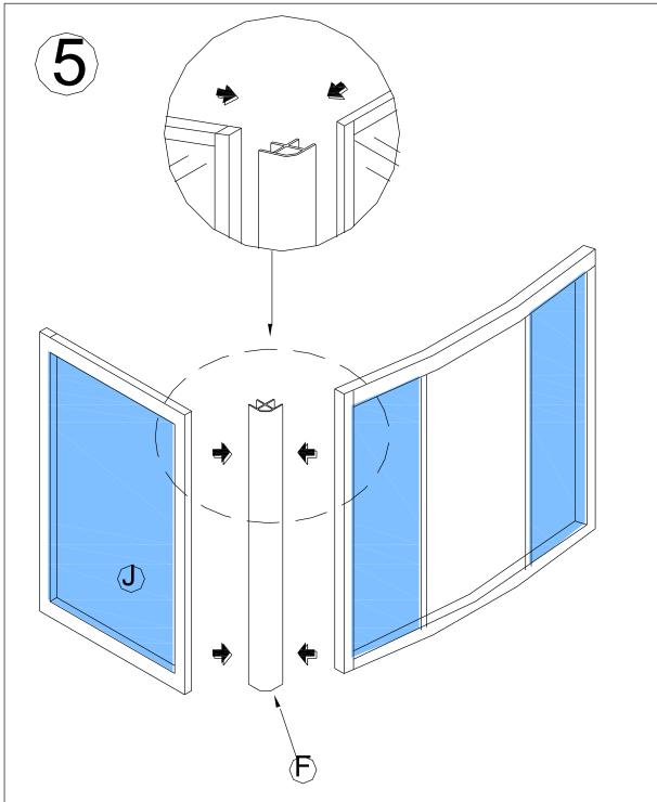
Connect the glass frame J with aluminum frame of the step 4, right to the groove of aluminum F.
