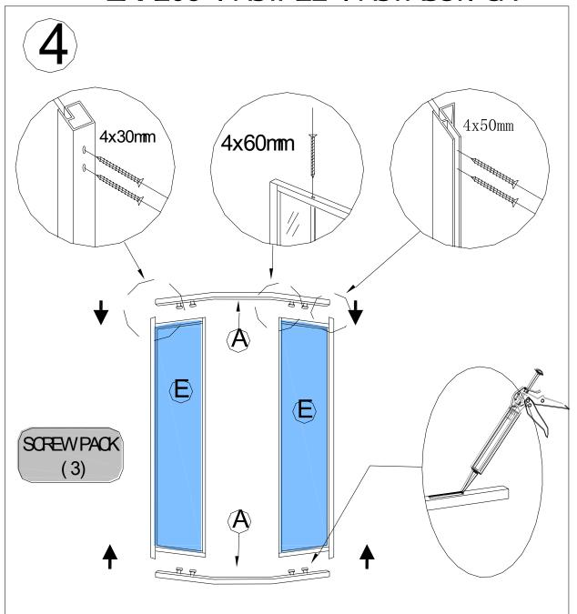
Fill the location of connecting orbit A and glass frame with sealant: make sure the screw holes of orbit are right to that of glass frame and fasten them with 4X30mm, 4X50mm, 4X60mm screws.
