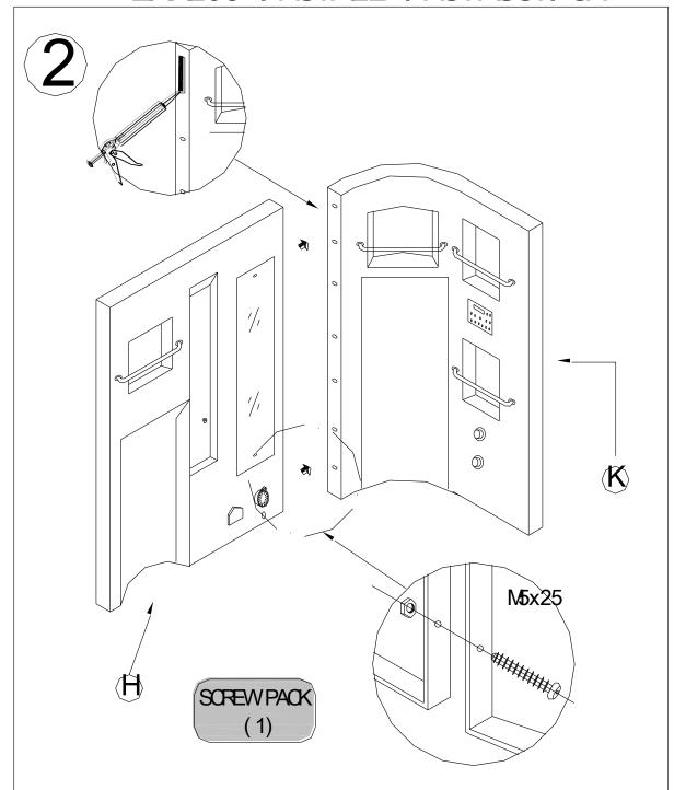
Connection of back and side panel: Fill the relevant section with silicone sealant; right to the screw holes and fasten them with 5X25mm screw with nut.
