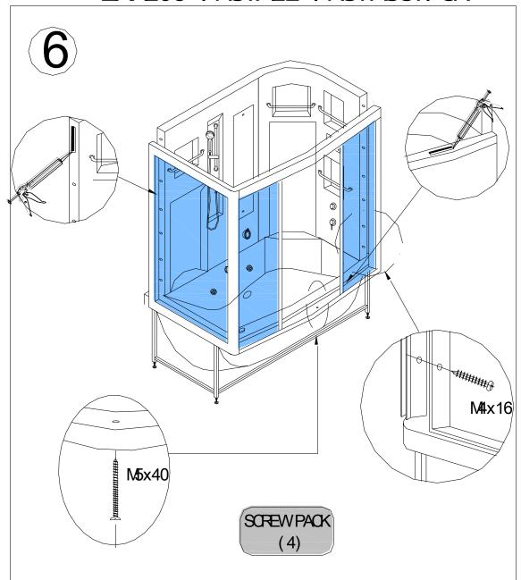
Put the front glass frame onto the massage bathtub, right to the holes of side panel and massage bathtub. Insert the groove of doorframe into the convex of side glass, fill with sealant or sealant strips and fasten with M5x40mm and M4X16mm screws.
