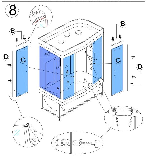
Refer to the drawing, fix the rubber strips B and D into the glass door C, then fix the door onto the cabin, adjust the screws and make sure the door sliding smoothly.
