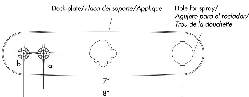
Note: Two options for screwing metal threaded rods.
